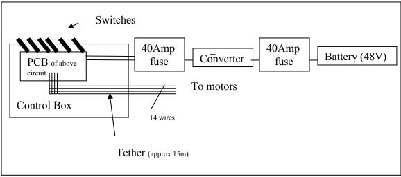
The system block diagram for this can be seen below.
