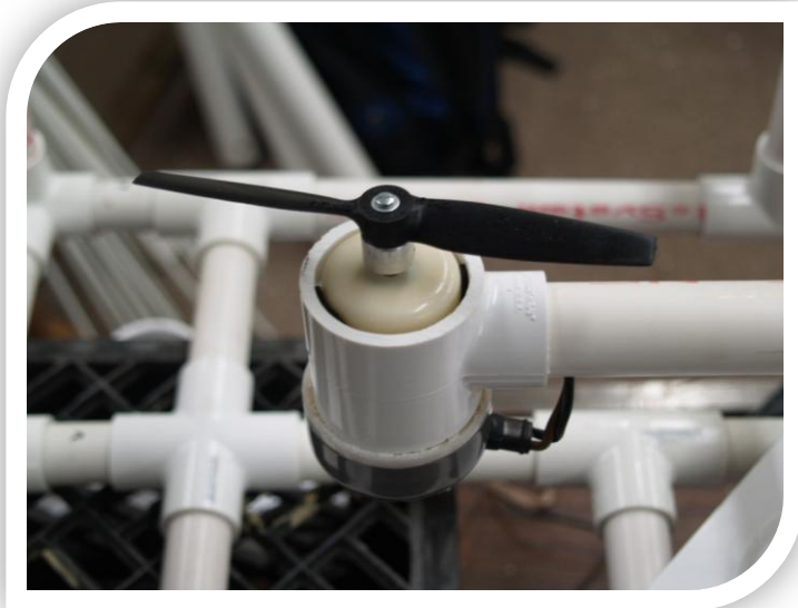
Figure 9: A close up of one of URSULA's thrusters.
