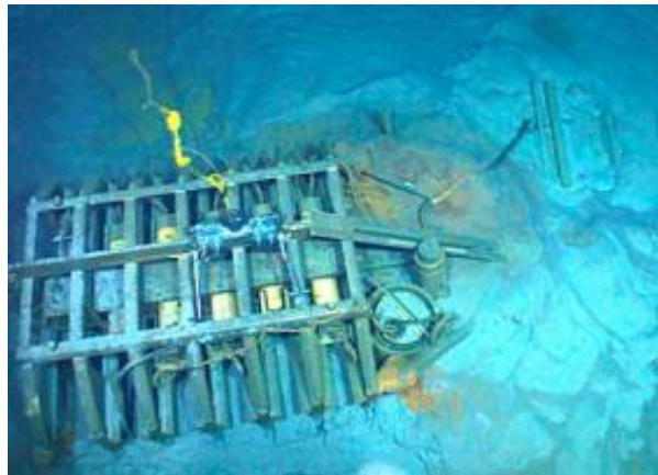
Figure The HUGO junction box almost ready to be retrieved from the ocean floor. The box monitored activity on Loihi Seamount
