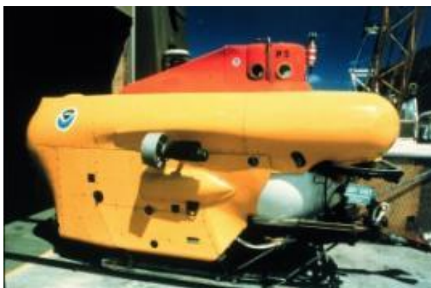
Figure Pisces V operated by NURP's Hawaii center dives to 2000 m
