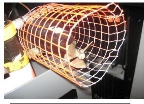
Figure 4: Safety Measure: Protection to Cover the Propeller samples of the crustacean. To accomplish all of these things, we have four motors: two are 3785 Lph bilge pump motors, mounted at the rear, and two are 4732 Lph bilge pump motors for vertical motion. Together, these cave. Each of the rear-facing motors is controlled independently, while the two vertical motors are controlled simultaneously; this allows for both a wide range of motion and a stable robot.
