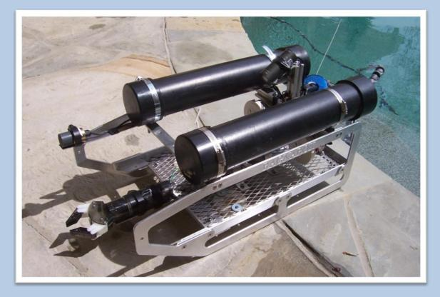
Name: *Ragnarok* Cost: \$2,596.04 Materials: Aluminum Sheet Metal Dimensions: 30.48 cm (Width) x 20.32 cm (Height) x 60.96 cm (Length) Weight: 8.2 kilograms Safety Features: Rounded off corners on all sides, fuses installed, foam on tether to prevent entanglement with propellers
