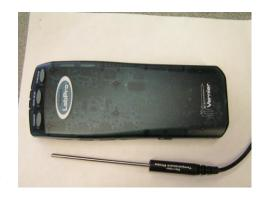
Figure 17: venier and temperature probe.
