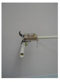
Figure 21: Task Specific device to pick up the PVC pipe, top view.
