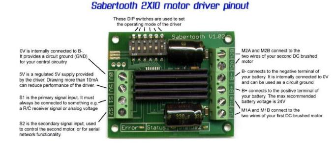
Figure 8: Sabertooth 2x10 motor controllers
