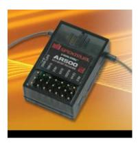
Figure 5: Remote Control Receiver
