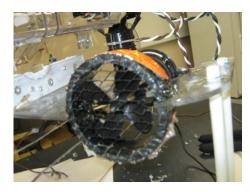
Figure 12: The epoxyed, mesh on the outside of the thrusters. 4-blade prop shown
