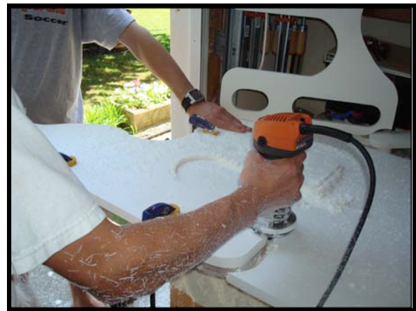
Figure 7: Using the router to transfer the frame template to LDPE. (Photo: Brennan)
