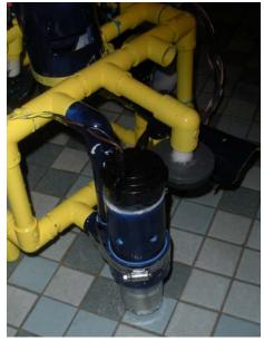
(Photo 11: the Suction Sampler)
