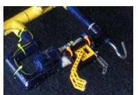
(Photo 8: Hook and gripper tool package)
