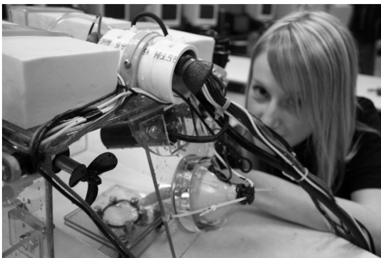
Team member Olivia Brown points out our homemade piezo crystal hydrophone. Did we mention it was homemade?
