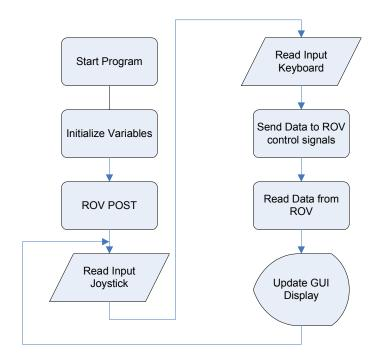
Figure 8 - Software Flow Diagram
