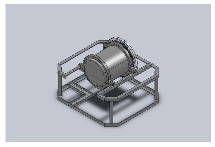
Figure 1 - ROV Chassis and Mass Properties
