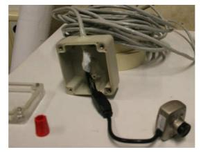
Fig 2.7 – Making of a water-proofed box with Rubber Tubing for Water proof function of the camera
