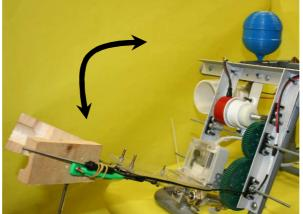
Fig 2.13 – Moveable pliers governed by a gear system and motor
