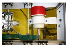
Fig 2.14 – Driving motor of the gear system
