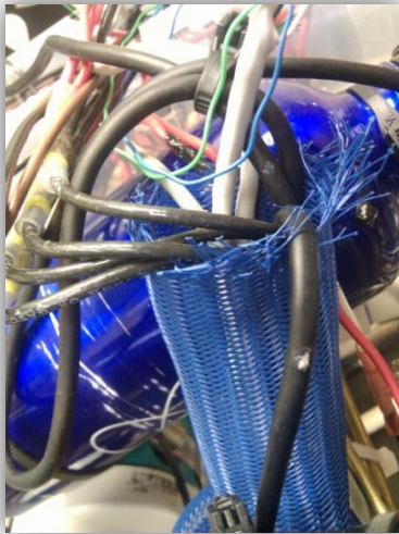
Figure 4 – CAT 5 cables and camera wires exiting the tether on the vehicle, routed to their corresponding systems.
