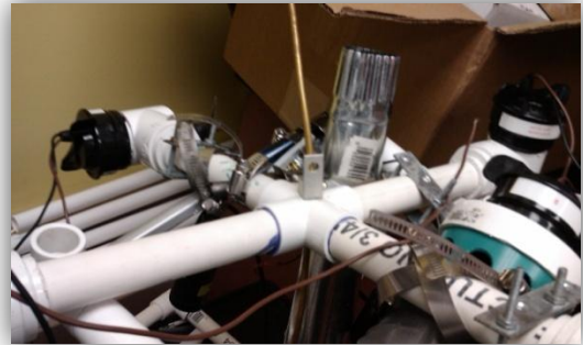
Figure 8 – Top portion of ROV frame with mission props and motors attached.
