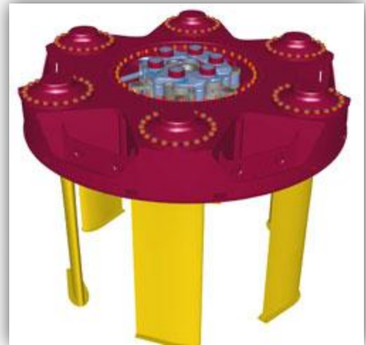
Figure 14 – Dual cycloidal drives, such as this Voith Schnieder Propeller, are capable of controlling all movement with the x,y plane with speed and precision.
