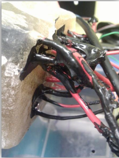
Figure 6 – The top of the relays, water sealed in epoxy with the extruding wires visible.
