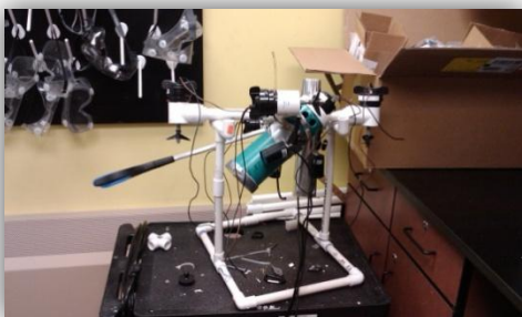
Figure 9 – The ROV under construction. Note mission components such as the grabber and vacuum.
