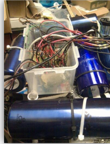
Figure 3 – The relays exposed in their plastic container, mounted at the top of the ROV.
