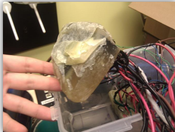
Figure 7 – The bottom of one water sealed relay setup, contained inside the plastic contained mounted on top of the ROV, ensuring little movement of intricate wiring setups during the mission.
