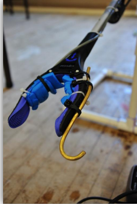
Figure 12 – The claw apparatus, with attached copper hook, used to manipulate various mission elements.
