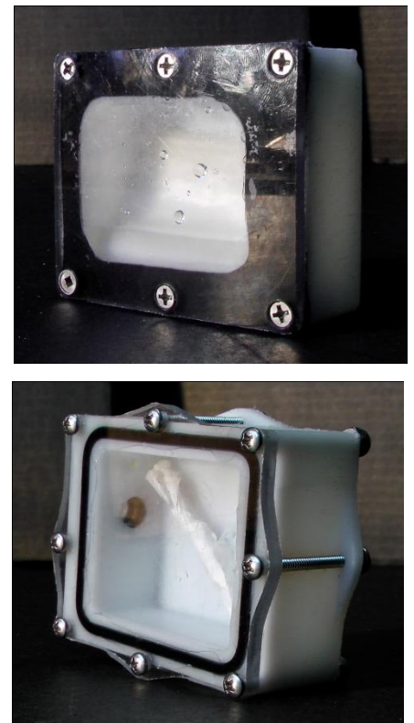
Figure 19. Leaky (top) and successfully waterproofed (bottom) servo boxes.
