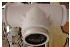
Figure 9: Front camera secured in PVC connector
