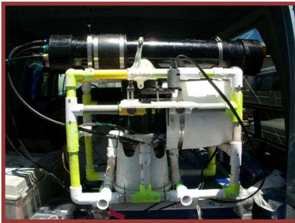
Figure 3 - ROV The Beast - Prototype - Used to test equipment and tools before attaching to competition ROV Rip Tide
