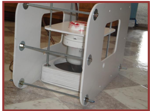
Figure 2 - ROV Rip Tide before payload items and buoyancy installed
