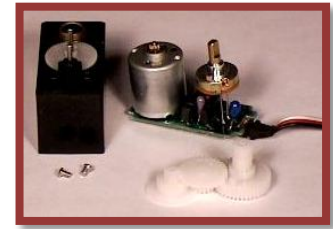
Figure 11 - Dismantled Servo -2.17mm x 20.1mm x 42.9mm
