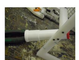
The temp probe is encased by a thin wall sink drain pipe to help position it correctly on the chimneys. The readings of the temp probe are taken using a CBL-2, which sends the data to be read to a scientific calculator, the Ti-84.
