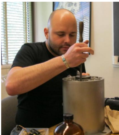
Figure 5: Arthur Aldridge filing away burrs on the waterproof connector holes.
