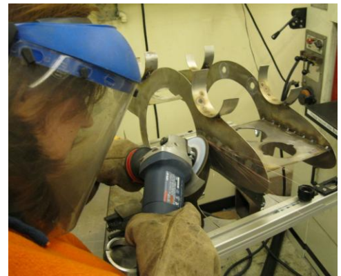
Figure 15: Kristine Summerfield grinding the ROV Chassis.
