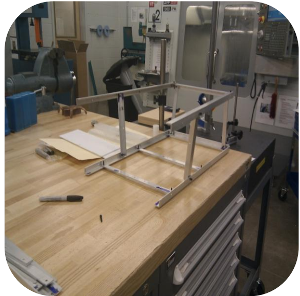
Figure 3.5 - The first time the main frame of the ROV was put together in the workshop (bolts not tightened)
