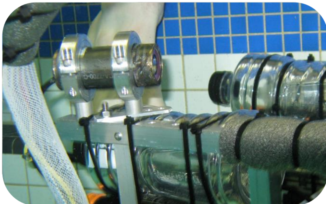
Figure 3.12 - Rear facing camera mounted on top of the ROV near the front (Note: Buoyancy in photo was temporary)
