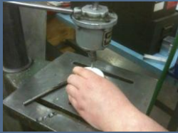
Making the delrin enclosures
