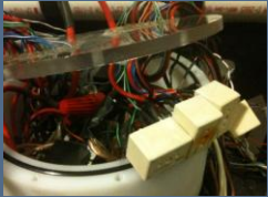
Sub-Sea Electronics Module with relays exposed
