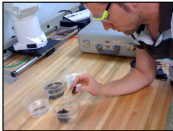
Figure 29. Nick Waterproofs a Servo in a Mineral Oil Bath
