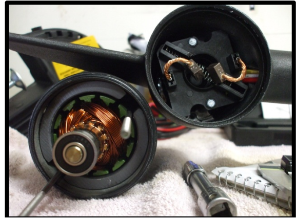
Figure 16: Trolling Motor sealing surfaces
