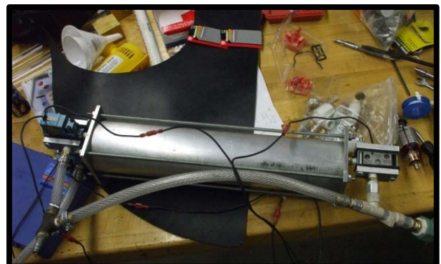
Figure 19: Dynamic ballast tank
