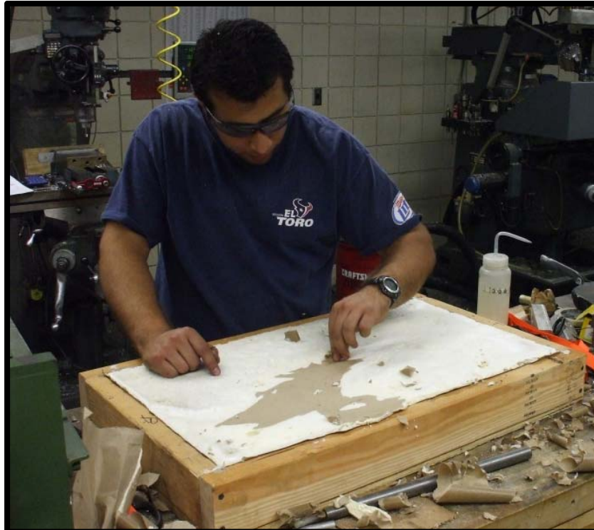
Figure 17: 2-Part Polyurethane static buoyancy in mold
