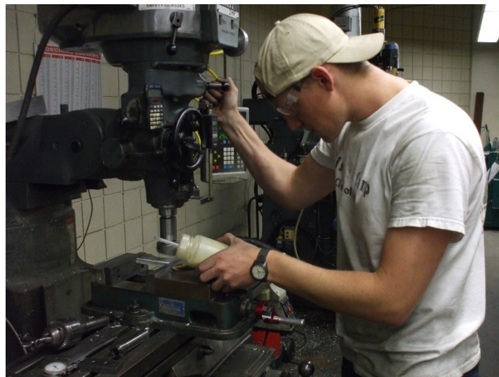
Figure 13: Milling Ballast tank mounts
