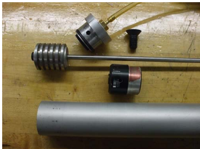
Figure 5: Fabricating 40.64cm stroke pneumatic actuator
