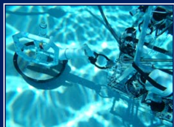
Removing the hose line from the top kill manifold and reinserting it into the well head.
