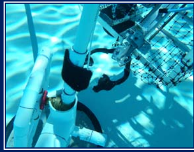
The manipulator cutting the pipeline.
