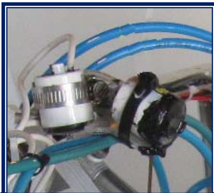
Close up of our two top mounted cameras
