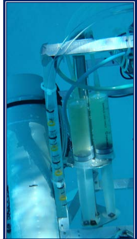
Our final Depth Sensor is mounted on the structure and based on air compression.
