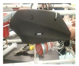
GPH bilge pump. Two 1100 pumps are used for forward and backward movement and the remaining two are used for up/down movement The single 700 pump is used to aid in reverse movement, which plays an especially important role in completing the valve wheel mission.
