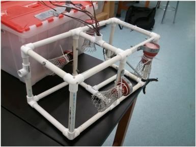
**Buoyancy:** We elected to keep the ROV neutrally buoyant, as many of the tasks of the mission required delicate and precise maneuvering that positive or negative buoyancy might interfere with. To offset the weight of the ROV, we used positively buoyant polyurethane and store-bought kickboards, and distributed it across the frame evenly to ensure neutral buoyancy.
