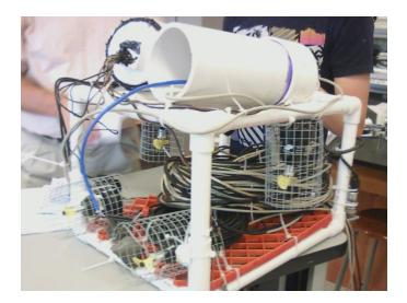
Special Features: We have a pressure sensor attached to our electrical board for measuring depth during Task 3. To manuver the robot we are using controllers which run in conjunction with our programmed electric board.
