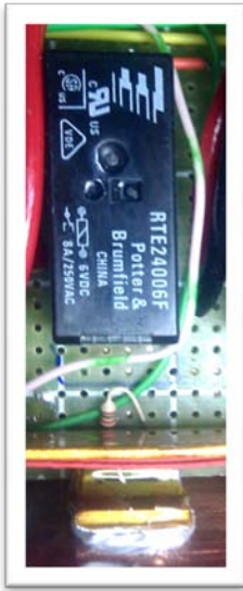
Figure 3: Relay and MOSFET combo
