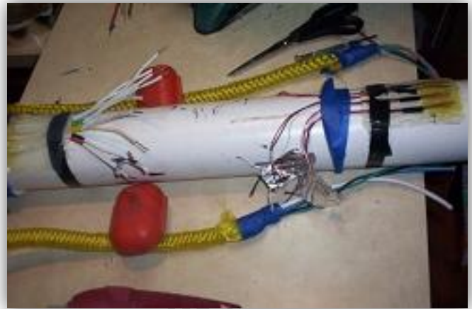
Figure 13- Pipe with wires fed in. This design was later abandoned.
