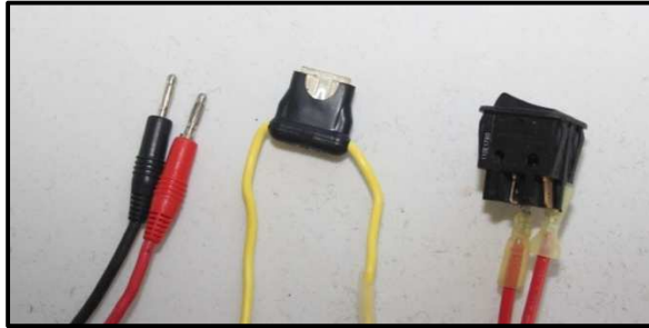
Figure 1-11: Banana leads, 25 amp fuse, and safety switch.
