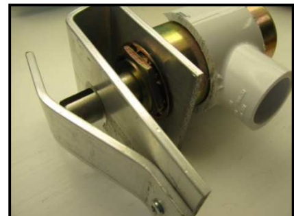
Figure 2-4: Solenoid Underwater Release System
