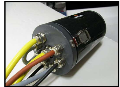
Figure 1-5: Water Tight Cylinder
