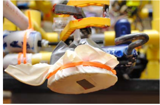
(Picture 11: Nozzle leading to the suction sampler, held in the gripper)
