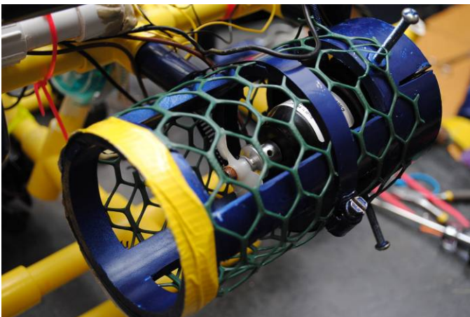
(Picture 4: Motor in shroud)
