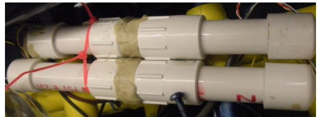
(Picture 2: Waterproof electrical connectors, sealed)
