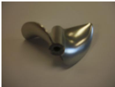
Figure 7: Top, Solidworks diagram of the propeller, bottom left, the off-the shelf propeller blade used in generation one of the ROV, bottom center, front view of our custom designed propeller blade, bottom right, side view of our custom designed propeller blade.
