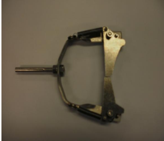
Figure 22.3: Photograph of the gripper that attaches to the U-bolt.
