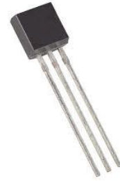
Figure 14: The DS18B20 is used as our temperature sensor.
