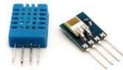
Figure 16: DHT11 acts as the humidity sensor, detecting water leakages in the electronics tube.
