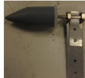
Figure 23: Photograph of the wellhead cap.
