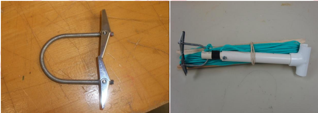
(Above Left: Tether Tool; Above Right; Our tool with the PVC extension and detachable U-Bolt with toggles.
