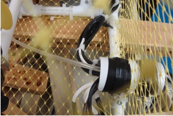
(Above: Tether restraint, located on the rear of the ROV)
