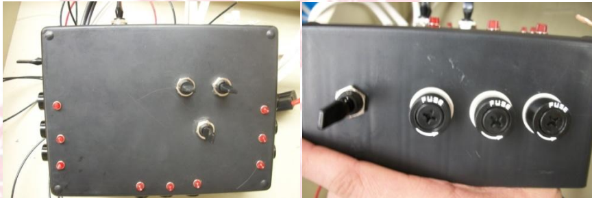
(Above-Left: Top View, ROV controller; Right: Left side Control Box, note fuse holders)
