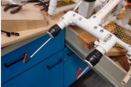
(PVC Hooks, used to grab the PVC ring and carry the well-cap)
