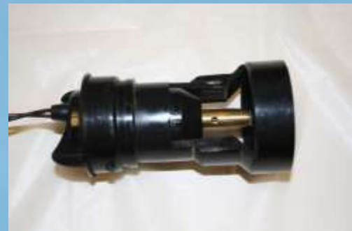
Figure 2. In house designed and fabricated thruster.
