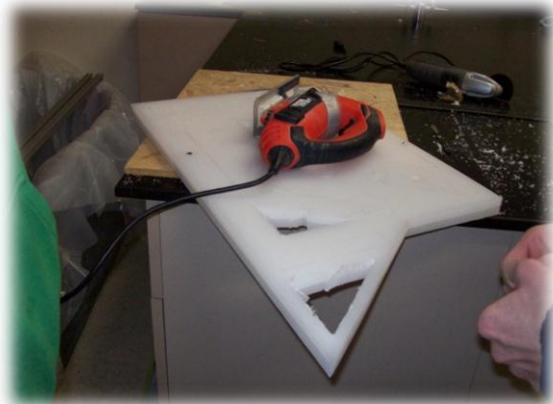
Figure 3 - Students cutting frame sides from LDPE
