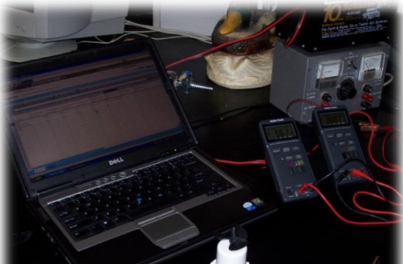
Figure 12 -Laptop and multimeters being used to measure current and voltage while motors are powered at different voltages
