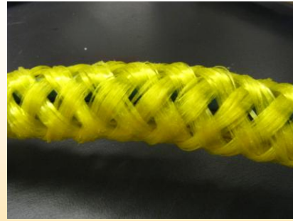
Figure 6: Tether covered with hollow braid rope for buoyancy
