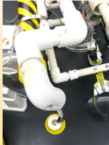
Figure 15: Sample collector holder on ROV
