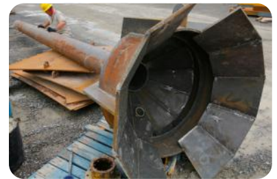
Fig 2.6 Top Kill Manifold (bp.com)
