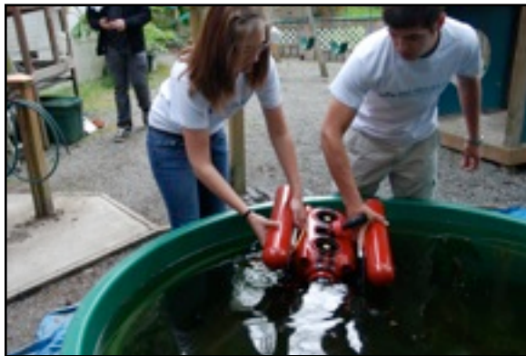
Figure 12 - Testing the ROV in a small tank
