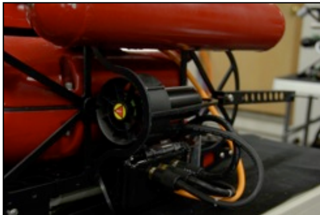
Figure 8 - The Seabotix thrusters attached to the machine
