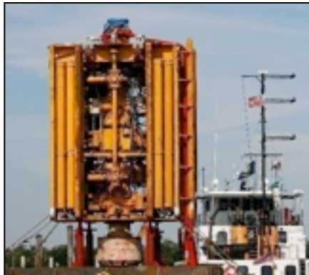
Figure 13 - The blowout preventer
