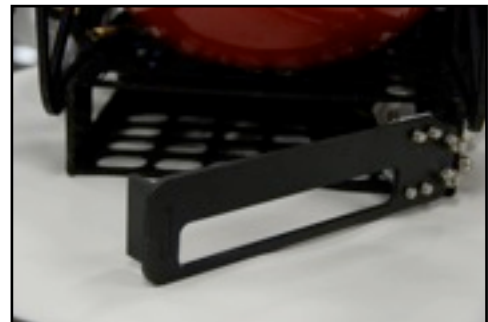
Figure 5 - The hinged door on the retrieval system
