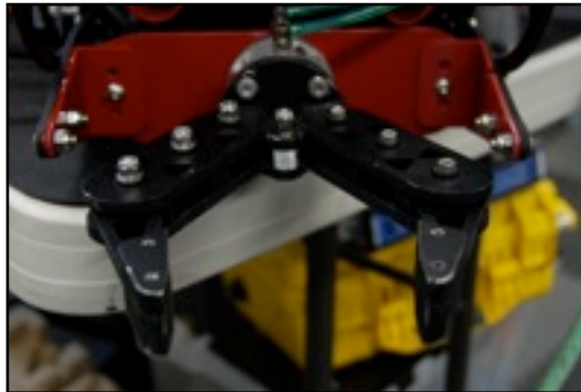
Figure 4 - The pneumatically-controlled manipulator
