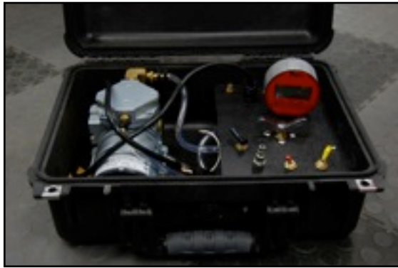
Figure 6 - The pneumatic control box with the pressure gauge installed
