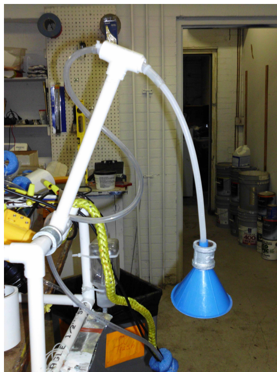
Figure 6: The funnel is placed at the end of the tube to ease collection of the water sample
