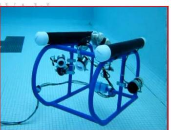
Features: Gripper/claw, liquid extractor, custom control system
