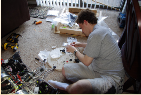
Fig. 6 - Lawrence Goldstein refurbishing the thrusters from Hybris
