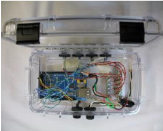
Figure 2.4.4: Otter box housing brain of the ORCA
