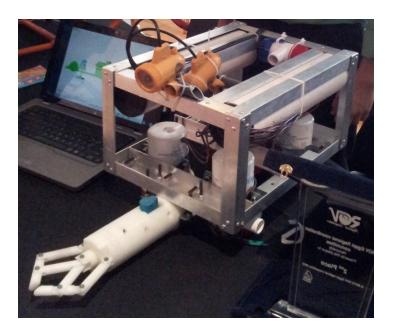
**Special Features:** Using bilge pumps for motion and well isolated tubes for on-board circuits.
