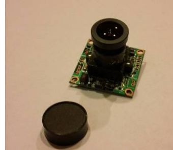
Figure 6: A not yet waterproofed board camera
