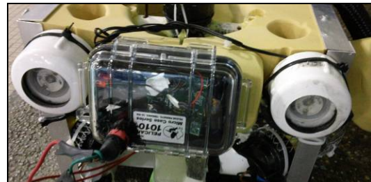
Figure 15: The metal detector mounted
