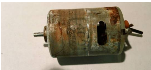
Figure 19: A corroded bilge pump replacement motor cartridge
