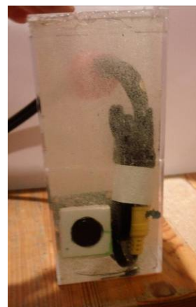
Figure 7: The main camera potted in epoxy
