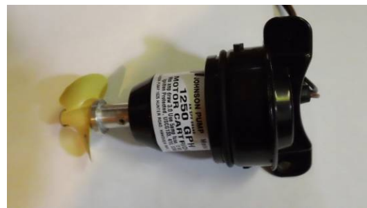
Figure 5: A bilge pump replacement motor cartridge
