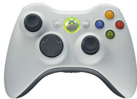
Xbox controller used to operate the ROV
