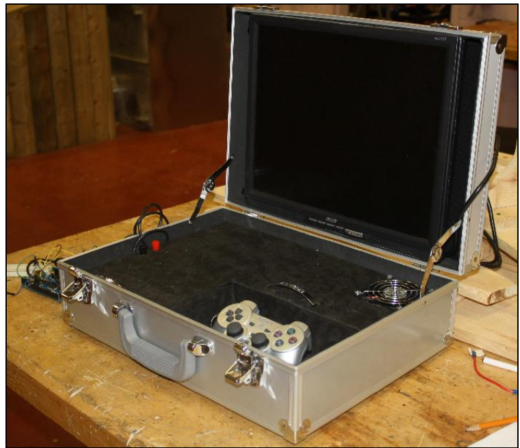
Figure 29- One of the control boxes with the monitor velcroed in
