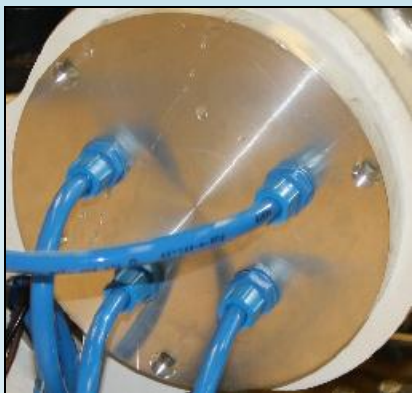
Figure 26- One of the end caps with the pneumatic tubes plugged in
