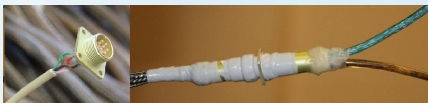
Fig. 16 "Quick Connector" and the final version of the basic socket.
