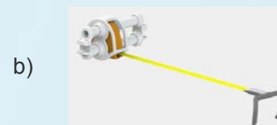
Fig. 11 Range finders: a) – laser rangefinder, b)- roulette with a flexible metal tape
