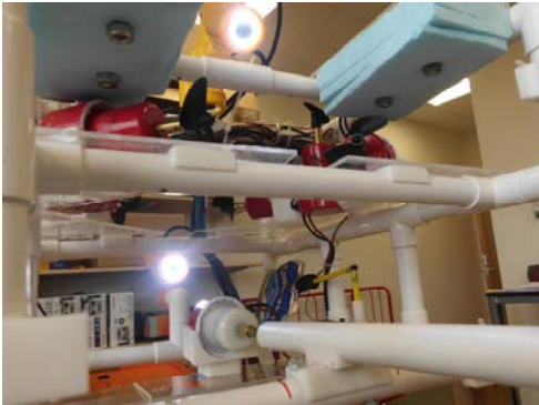
View from the front of SCOTIA, showing the three cameras. These give views of the area in front of the ROV, the frontal manipulator and spear, and magnetising device on the underside.
