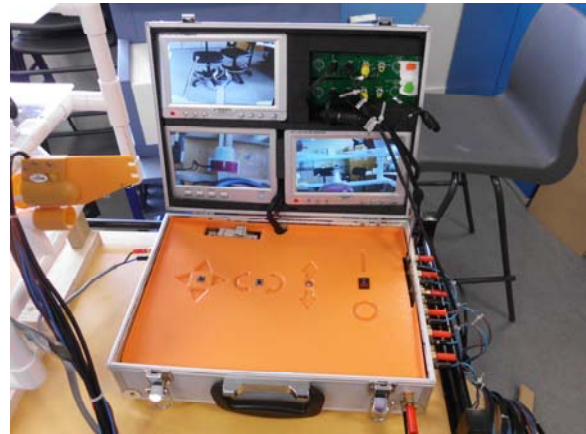
Main control suite (control circuit housed within)
