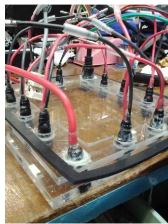
Installation of the plugs
