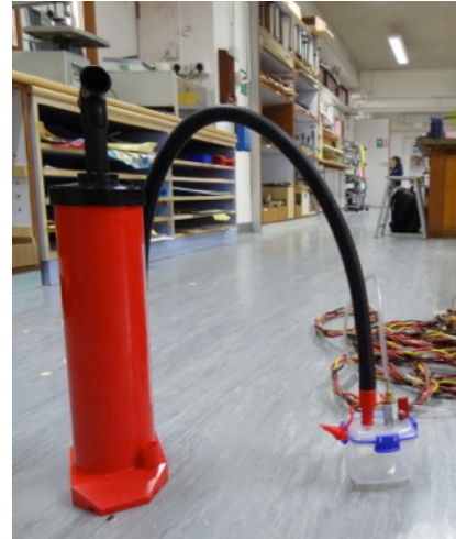
Figure 4: The pump (left) and reservoir (right) to collect a fuel sample.
