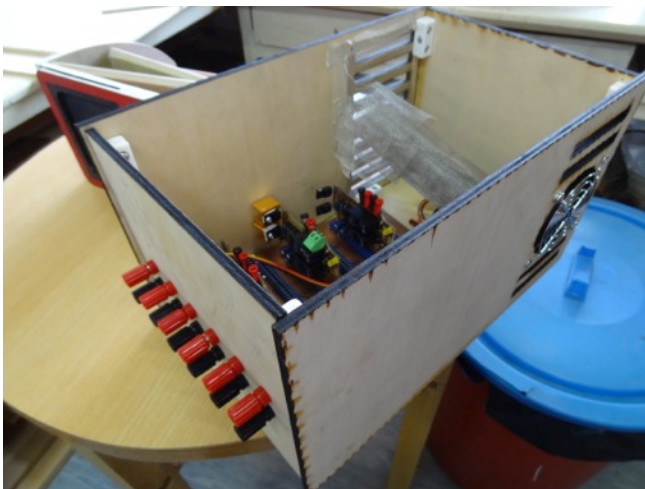
Figure 13: Image of the Motor Control Box
