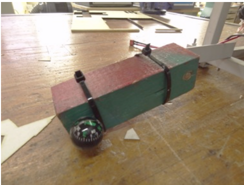
Figure 2: Compass used for determining ship orientation and metal detecting
