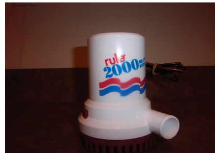
Bilge pump used for thruster motor
