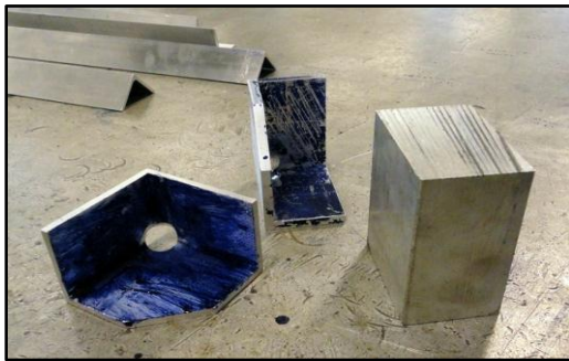
A before and after view of the aluminum blocks used in fashioning corner pieces for the ROV frame.
