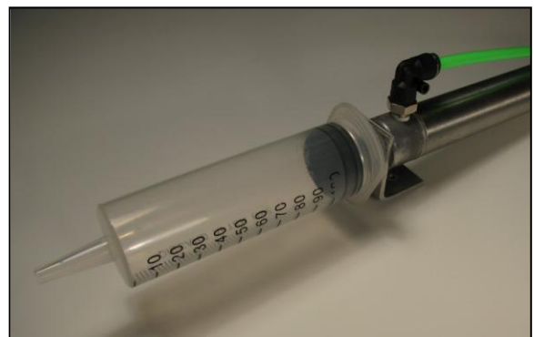
Figure 2-5: Oil Sample Retrieval System.
